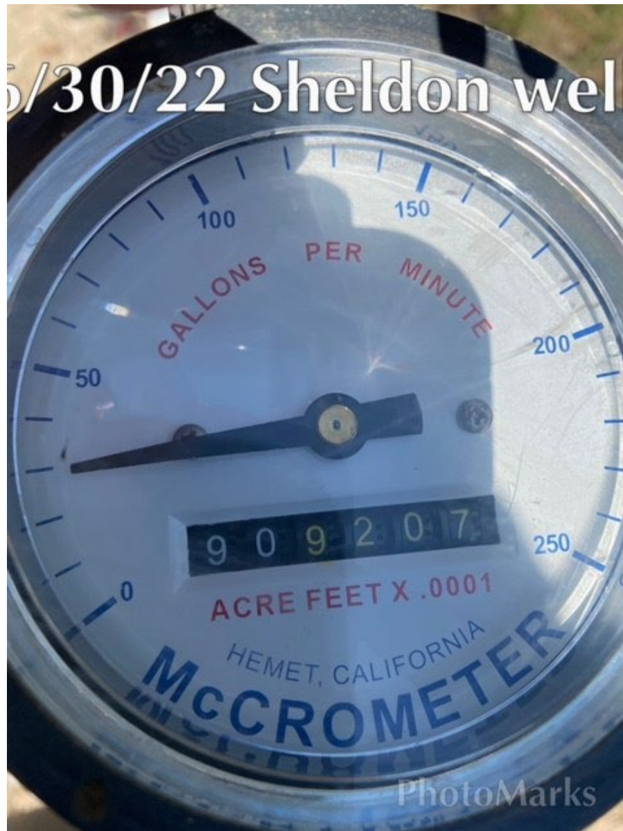
Photo 2. Example photo showing flowmeter face with totalizer digits and units visible and legible for compliance with Well Registration Form Item No. 6(d)(vi)(2).
