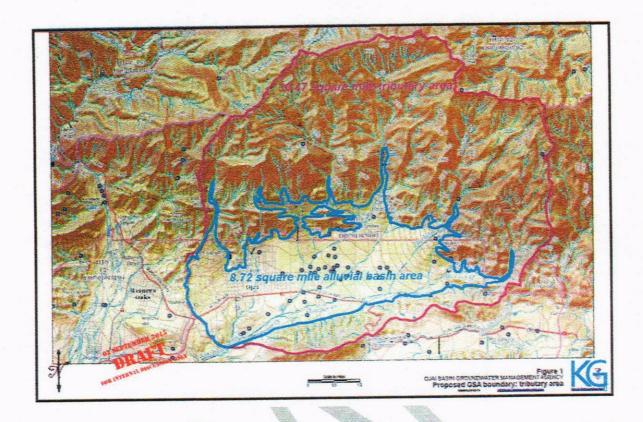
This map depicts the tributary area for the Ojai Basin. All 30.47 square miles drain toward the basin and contribute to the recharge of the basin; some groundwater within bedrock areas also contribute to alluvial basin recharge and supply water to wells. The GSA Boundaries should include recharge areas shown hereon.
